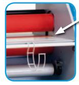
**Opening of the rollers** The 25 mm (1") maximum opening of the rollers enables the most common mounting operations.
