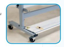
Feeding tray The graduated feeding tray is removable. While loading the film or print reels, it can be stored on the machine base without being damaged.
